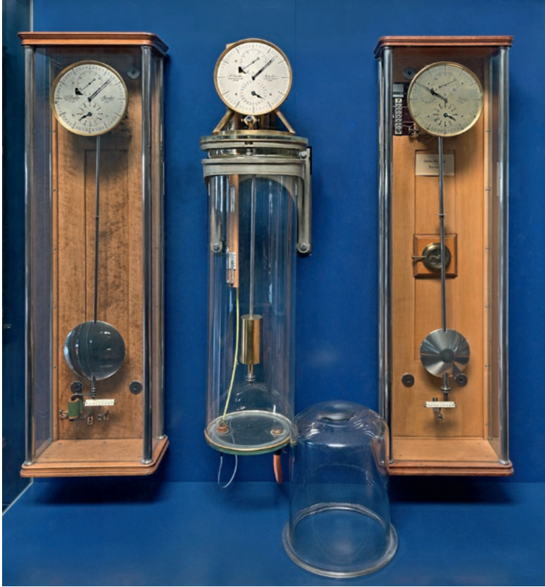
Fig. 12: Time-keeping system in the Deutsches Museum with master clock no. 98 in the glass tank and two slave clocks (Photo: Jürgen Ermert.-Deutsches Museum)
